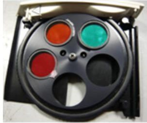
Figure 5.3: Customized filter wheel ensuring no light leakage around the filters.
