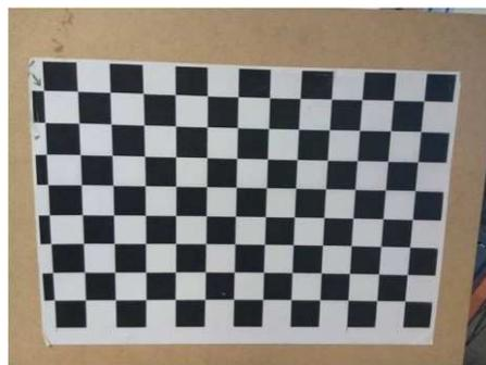
**Figure 4-5:** Camera calibration target
