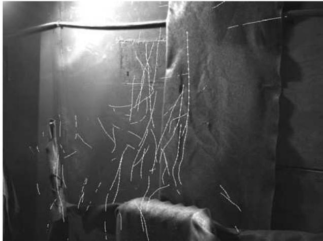
**Figure 1-10:** PTV measurement over a heater in a room [27]
