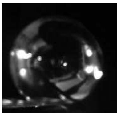
**Figure 1-3:** Single helium filled soap bubble. Light scattered on the shell can be seen. [54]
