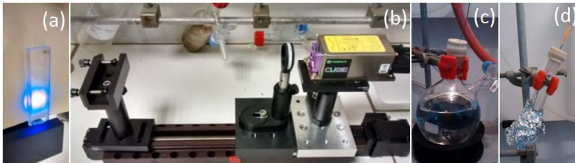
FIGURE 4.5: (a) The sample holder and the empty cell with laser spot on it, (b) experimental setup: sample holder, the lense of 50 mm to focus the beam and 404 nm continuous laser, (c) degassing of the acetonitrile, (d) mixing the powder and the solvent.
