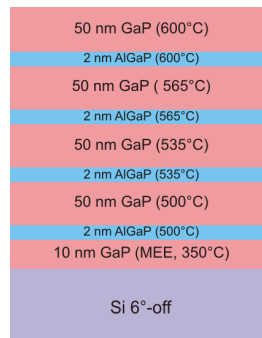
Figure 4.31 Sketch of the growth procedure of S1477
