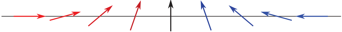
FIGURE 1.10: Scheme of a TW in a 1D system. The colors indicates the magnetization direction along the z axis.
