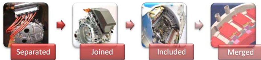
Figure 1.4 Different integration levels in mechatronic systems (Penas, Plateaux, Choley, & Rivière, 2009)
