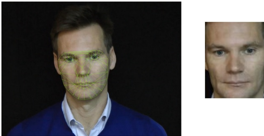
Figure 5-2: Example of face cropping: (left) a frame annotated with the detected landmarks, and (right) the cropped and aligned face region.
