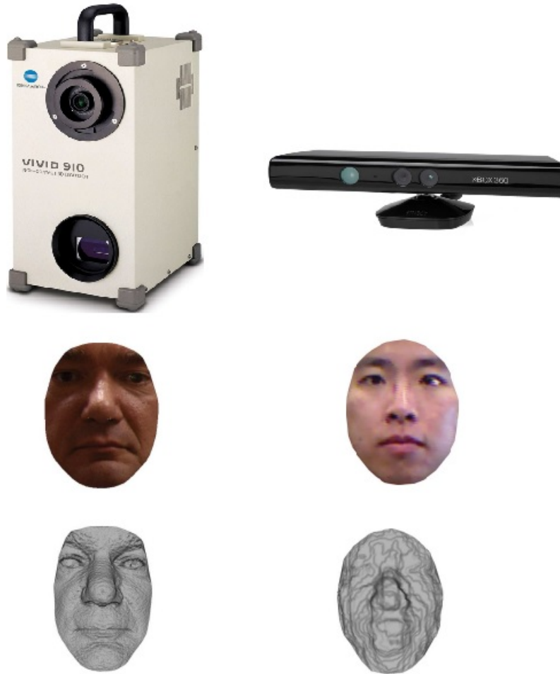
Figure 4-1: Comparing face images acquired with Minolta VIVID 910 scanner (left) against Kinect (right).
