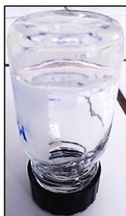
Figure 31: Hydrogel of trehalose monoerucate in water (5 wt%)
