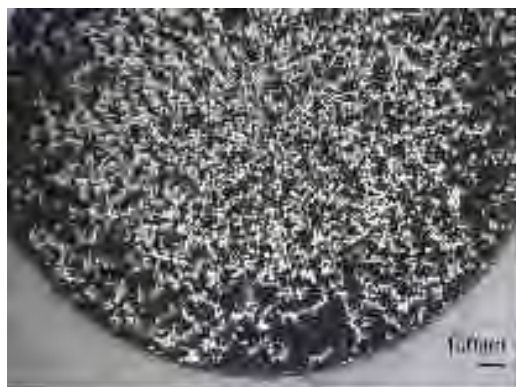
Figure 5 : Perovskite/carbon thin layer on glassy carbon observed by optical microscopy
