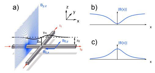
Figure 1.7: Dimple trap of two crossing wires. a) shows the current, wire and bias field configuration with the resulting field in the y-z plane. The field strength minimum is shown as a black line, the minimum line for  $I_1 = 0$  is shown as the dashed line. b) shows the potential along x for  $I_1 > 0$ . c) shows the potential for  $I_1 < 0$  and  $B_{0,x} = 0$  used for the H,U and Z traps. Adapted from [109].
