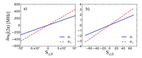
Figure 2.5: a) Shows the cavity shift given by Eq. A.1.1 for an effective atom number  $N_0 = 2 \cdot 10^4$ ,  $w_0 = 13.4 \,\mu\text{m}$  and L=1.2 mm for the two transitions possible with the resonator mode. b) shows a zoom to the central part, spanning the standard deviation of the shot noise  $(S_{z,0,max} = -S_{z,0,min} = \sqrt{\Delta S_{z,0}^2} = \sqrt{S_0/2})$ . The reduction of 3/4 from the mode overlap is taken into account (see Eq. 2.4.2).
