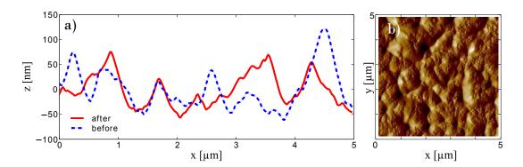
Figure 5.15: Au surface after RIE etch. The electroplated gold surface was measured before and after reducing the gold layer thickness by  $\sim 350\,\mathrm{nm}$ . a) shows a cut along x of a measured 2D profile as shown in b). The measurements were performed on the same position on the chip and show with  $\sigma_{r,before} = 33.7\,\mathrm{nm}$  and  $\sigma_{r,after} = 32.3\,\mathrm{nm}$  no increase of the surface roughness during the etch process.
