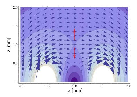
Figure 5.10: Magnetic field of two wires with a parallel current I=1A and a distance of 2 mm between the two wires. In addition to the vector field, the magnetic field magnitude  $|\vec{B}|$  is shown as contours with dark blue for  $|\vec{B}| = 0$  G up and white for  $|\vec{B}| > 5$  G. The red arrows show the direction of the field gradient along z above and below the magnetic field maximum along z.
