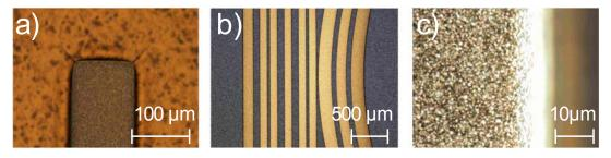
Figure 5.19: Microscope pictures of the science chip. a) shows the cracking of the photoresist during the electroplating as fine diagonal lines in the wire corners. b) shows the wires in the trapping region. c) shows a close-up of a science chip wire edge, where the granularity of the electroplated gold is visible.
