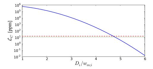
Figure 4.3: Clipping loss for finite mirror diameters (blue line). The clipping loss is reduced by increasing the ratio of the mirror diameter to the beam radius on the mirror. For comparison, the red dashed line indicates the expected absorption loss  $\mathcal{L}_A = 15\,\mathrm{ppm}$  and the green dotted line the expected scatter loss  $\mathcal{L}_S = 11\,\mathrm{ppm}$  at 780 nm.
