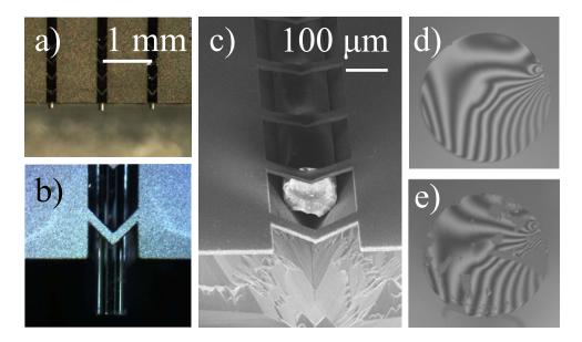
Figure 3.8: Microfabricated nickel clamps. a) and b) show microscope images of fibers  $(\emptyset = 125 \,\mu\text{m})$  held by nickel clamps. c) shows a SEM picture of the Si v-groove with a non-cleaved fiber. d) shows a fiber facet before and e) after inserting it into a groove with nickel clamps, showing debris accumulated on the surface.
