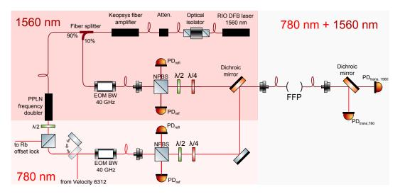
Figure 4.16: Laser setup for 780 nm and 1560 nm. Light at 780 nm and 1560 nm can is coupled simultaneously to the FFP resonator. With the flip mirror we can choose between the widely tunable velocity laser, or use the frequency doubled light. Using components of the free optical component library of [200].
