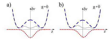
Figure 1.4: Mean field and second order Zeeman shift. a) shows the near cancellation of the total shift (solid black line) by the addition of the negative mean field shift (dotted red line) and the positive second order Zeeman shift (blue dashed line) in zero gravity. b) shows the same situation including the gravitational sag (cf. Sec. 1.4.4). Adapted from [97].
