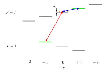
Figure 1.5: Zeeman sub-level diagram of the  $5^2S_{1/2}$  manifold of  $^{87}\mathrm{Rb}$ . The degeneration of the hyperfine levels is canceled by an external quantization magnetic field and the Zeeman sub-levels are visible (grey lines). The clock-states used in TACC are marked green and the RF (MW) transition is indicated by a blue (red) arrow.
