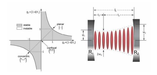
Figure 4.1: Stability diagram and resonator configuration. Taken from [135].
