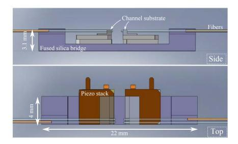
Figure 4.19: Bridge design. The fused silica bridge is shown with sheer piezo stacks glued to it. In the top view the electrodes of the piezo stack can be seen. On top of the sheer piezos the channel substrates are glued, which hold the fibers.
