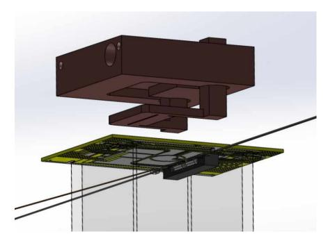
Figure A.8: Macroscopic U with chip assembly (cf. Sec. 5). Shown is the macroscopic U, which lies inside a copper block for water cooling. The small groove in the U center allows to place a wire of  $\emptyset = 0.5 \,\mathrm{mm}$ , which is named "macroscopic I".
