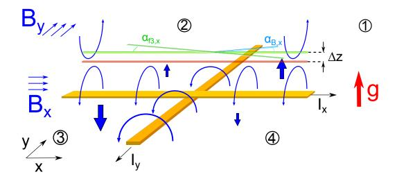
Figure 1.10: Gravitational sag in a dimple trap. The red line marks the center of the 2D-quadrupole trap created by the current  $I_x$  and  $B_y$ . The green line marks the potential minimum taking gravity into account. As this position is above the zero line of the magnetic potential, the bias field along y dominates over the wire field and the residual magnetic field at the trap position has an additional component along y.
