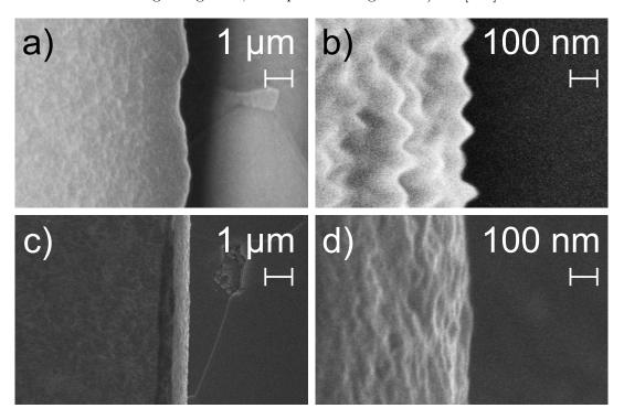
Figure 5.18: SEM pictures of SC wire edges. On all pictures the gold surface is on the left. a) shows the first attempt, where the edge of the chip wire shows irregularities of  $\sim 1 \,\mu\mathrm{m}$  due to problems with the photoresist development. b) shows an old chip of the previous TACC chip production [231] declined by 50°. c) and d) show the wires of the final TACC 2 science chip before RIE etching without inclination.
