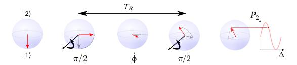
Figure 1.3: The Ramsey sequence depicted on the Bloch sphere. The grey (red) arrows depict the state before (after) the manipulation of each step. The speed of the dephasing is given by  $\dot{\phi} = 2\pi\Delta$ . Figure adapted from [89].
