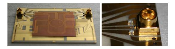
Figure 5.17: Chip assembly with MW connector and bias-tee capacitors soldered and the SC glued to the base chip.
