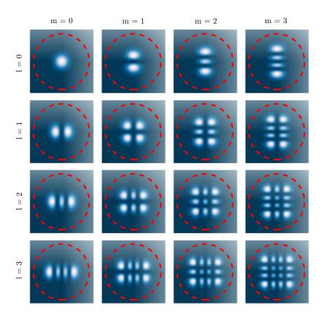
Figure 4.9: Intensity distribution of the Hermite-Gauss modes on a cavity mirror of a cavity with length L=1.22 mm and ROC R=1.56 mm. The edge length is  $130\,\mu m$ . The red circles indicate a clipping radius of  $r_{clip}=58\,\mu m$ .
