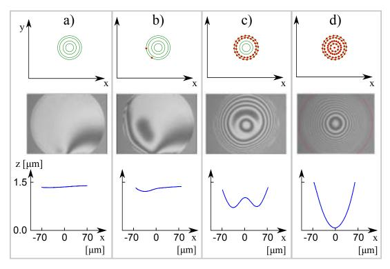
Figure 3.16: Multi shot sequence. The first row shows the shot positions, the second interferograms of the fiber facet and the third a cut along x through the 3D profile at y=0. The different columns show the fiber facet after a) 0, b) 2, c) 40 and d) 69 shots. After inspection the shape can be fine tuned with an additional shot of reduced pulse length to the center.
