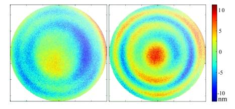
Figure 3.4: Residual depending on profilometry position. The same surface was scanned twice with a distance offset of  $\lambda_P/8$  and fitted with a 2D-paraboloid, the edge length is  $60\,\mu\mathrm{m}$ . The residuals shown have a sinusoidal modulation, dependent on the initial profilometry position. Averaging two profiles with such a distance offset reduces strongly the spurious effects of the reconstruction algorithm.
