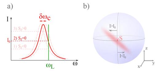
Figure 2.3: Cavity feedback squeezing. a) The cavity resonance is depicted in red for three different values of  $S_z$  (1:  $S_z < 0$ ; 2:  $S_z = 0$ ; 3:  $S_z > 0$ ) shifting its frequency with respect to a laser of fixed frequency  $\omega_L$  shown as a green vertical line. b) the circular uncertainty region of a CSS is sheared on the Bloch sphere, creating a squeezed spin state.
