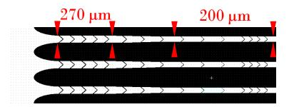
Figure A.1: Mask layout for nickel clamps for fibers of  $\emptyset = 125 \,\mu\text{m}$ . The black region marks the position where later nickel is grown. The wider groove on the left allows to push the fiber in and holds the copper coating with the first 5 clamps.
