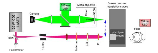
Figure 3.2:  $CO_2$  dot milling setup: Precision translation stages are used to control the  $CO_2$  beam position on the fiber and to translate the fiber to the optical profiler position for surface characterization. Light coupled into the fiber core allows a precise centering of the mirror profile. The  $CO_2$  focusing lens (FL) is a  $f=25\,\mathrm{mm}$  asphere illuminated with a beam diameter of  $7\,\mathrm{mm}$ .
