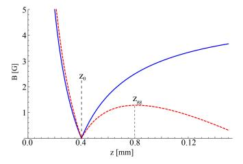
Figure 1.9: Effect of gravity on trap depth. Shown is the magnetic potential for a trap as in Fig. 1.6 with I=1 A and  $B_0 = 5$  G as the blue line. Taking gravity into account (red dashed line, gravity points along z), the effective potential the atom sees is modified.
