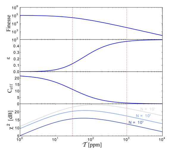
Figure 2.7: Influence of the mirror transmission  $\mathcal{T}$  for a mirror loss of  $\mathcal{L}=30\,\mathrm{ppm}$ , a typical value for double-wavelength coatings.  $\epsilon$  converges to 0.5 assuming a read out on only one side of the resonator and no additional photon loss. The resonator mode waist used is  $w_0=13.5\,\mu\mathrm{m}$ , the atom cloud diameter  $\sigma=6.9\,\mu\mathrm{m}$ . The red dashed lines indicate the values chosen for our experiment (see Sec. 4.2.8).
