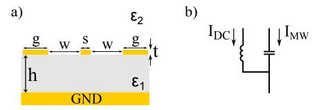
Figure 5.11: Coplanar waveguide and bias-tee
