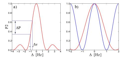
Figure 1.2: a) Rabi pulse following Eq. 1.1.3 with  $\Omega_R = 1$  and  $t = \pi$ . For  $\Delta = 0$ , the atomic state is fully transferred to  $|2\rangle$ . A pulse realizing the full transfer is referred to as a  $\pi$ -pulse. b) Comparing the spectroscopic response of the Rabi pulse from a) (red) with a Ramsey sequence (blue) with the same duration  $T_R = \pi$ .
