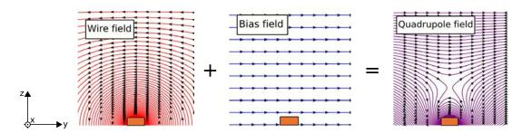
Figure 1.6: Basic principle of wire traps. Taken from [91].
