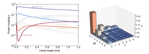
Figure 4.11: Higher order mode coupling. The graphs show the coupling of the fiber mode with waist  $w_f = 5.3 \,\mu\text{m}$  and a collaps length of  $L_{col} = 60 \,\mu\text{m}$  to the first few higher order modes of a cavity with a ROC of  $R = 1.56 \,\text{mm}$ . The transverse misalignment is  $d_x = 2.6 \,\mu\text{m}$  and  $d_y = 2.7 \,\mu\text{m}$ . On the left the length of the cavity is varied, on the right the coupling is shown for the cavity length  $L = 1.22 \,\text{mm}$ .
