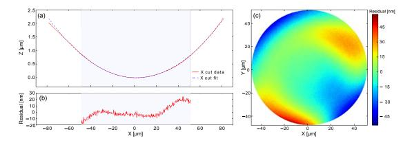
Figure 3.18: (a) Cut along the x-axis of a spherical profile on a  $220 \,\mu\text{m}$  diameter MM fiber and corresponding cut of a two-dimensional spherical fit  $(R=1475 \,\mu\text{m})$  on a circular region with a diameter of  $100 \,\mu\text{m}$ . (The shaded area in (a) and (b) indicates the fit region.) (b) Cut along the x-axis of the fit residuals. (c) 2D fit residuals.
