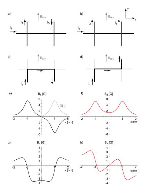
Figure 1.8: H/U/Z-trap. The left column shows the generation of a quadrupole trap with three wires (a)) or one wire (c)) and a bias field. The right column shows the generation of a IP trap with three wires (b)) or one wire (d)) and a bias field. e)-h) shows the calculated magnetic fields along x and z for  $B_y = 10 \,\text{G}$ ,  $I_1 = I_2 = I_3 = 2 \,\text{A}$  and a wire width of  $50 \,\mu\text{m}$  and a distance of the wires along y of 2 mm. Taken from [102].
