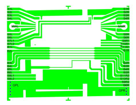
Figure A.7: Labeled base chip (cf. Sec. 5.2).
