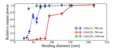
Figure A.3: Bending loss of large mode area PCF (cf. Sec. 4.1.6). The transmitted light was measured for the LMA15 and LMA20 from NKT photonics. A strong dependency of the bending loss on wavelength and effective mode field diameter can be seen. Bending diameter  $d < 160\,\mathrm{mm}$  should be avoided to exclude bending loss for the LMA20 at 780 nm. For this reason, we recommend to investigate the fiber-resonator mode coupling with the LMA15 for future large FFPs.
