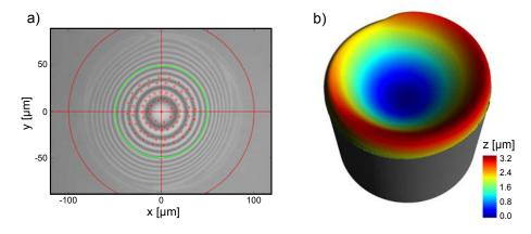
Figure 3.17: Large spherical surface machined on a  $200\,\mu\mathrm{m}$  diameter SM fiber. a) Interferogram of the surface after processing. The red circle shows the initial fiber diameter, the green circle shows the area over which the structure was optimized. The crosshairs indicate the center of the fiber. The red circles indicate the positions of the  $CO_2$  pulses. b) Surface profile measured by phase-shifting interferometry. (The grey area was added to indicate the fiber orientation.)
