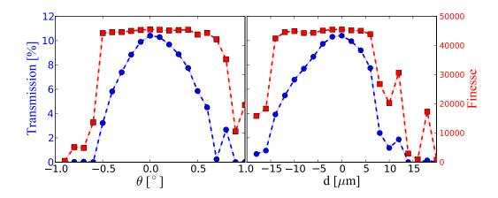
Figure 4.21: Simulated effects of misalignment. For the simulation the profiles and mirror losses of Fig. 4.5 are used at a cavity length  $L=1.2\,\mathrm{mm}$ . The fiber waist is  $w_f=8.2\,\mu\mathrm{m}$ . In a) the output mirror is tilted, in b) displaced. The blue circles mark the transmission, the red squares the finesse.
