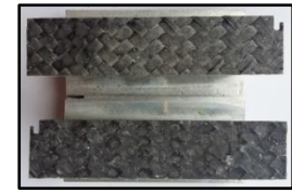
SP498/Prepreg fracture for \gamma=0^\circ
