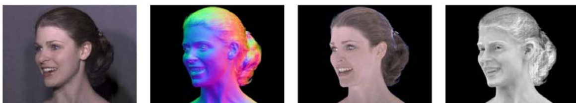
Figure 2.9 – Results from [WGT+05a], from the left to the right: input frame acquired with the acquisition setup, result Normal Map, albedo, ambient occlusions.
