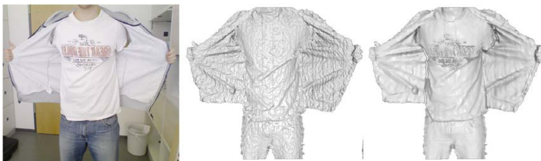
Figure 2.12 – Results from [WZN + 14], from the left to the right: RGB aligned image, input raw depth map, refined depth map.
