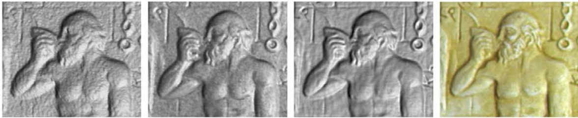
Figure 2.10 – Results from [NRDR05], from the left to the right: Rendering of 3D scanned range image, same scanned geometry, augmented with a measured normal-map (from photometric stereo), hybrid surface reconstruction, which combines both position and normal constraints, photograph.
