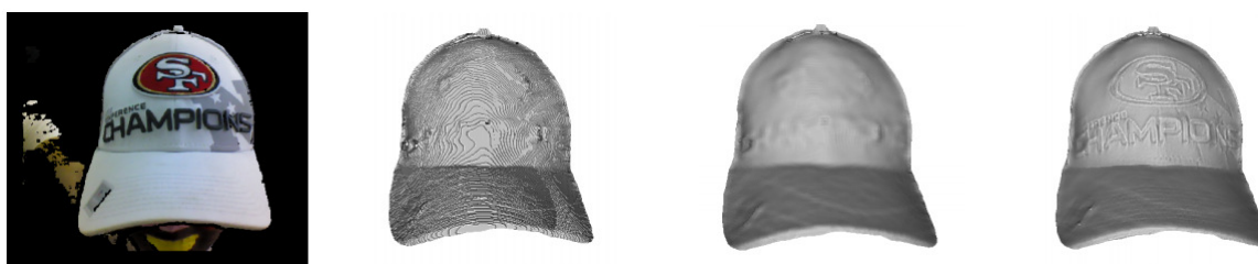
Figure 2.13 – Results from [OERW + 15], from the left to the right: RGB aligned image, input raw depth map, bilateral filtered depth, refined depth map.
