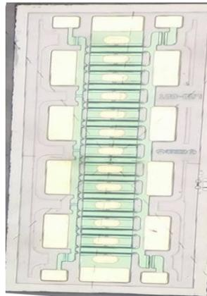
*Figure IV.38: Photo of the CGHV1J025D GaN Transistor Die*
