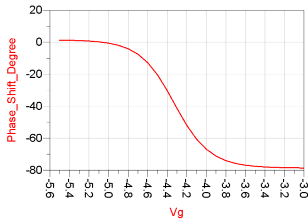
Figure IV.29: Phase Shift versus DC Bias at 10 GHz
