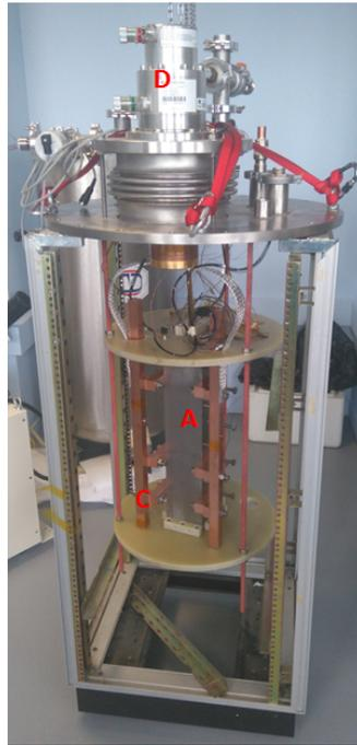
Fig. III.27 – MgB<sub>2</sub> measurement workbench with the magnet in A, the thermal parts in C and the cryocooler head in D.
