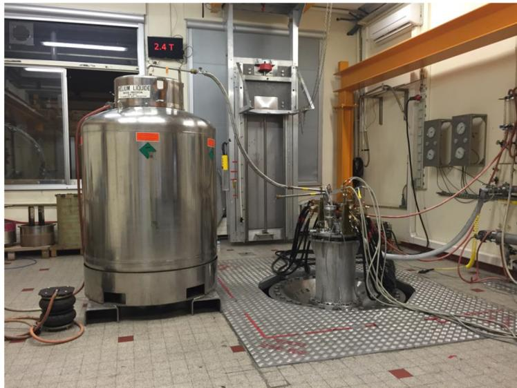
Fig. III.24 – MgB<sub>2</sub> critical current measurement setup.
