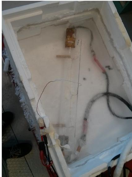
Fig. II.15 – Sample in the nitrogen bath.
