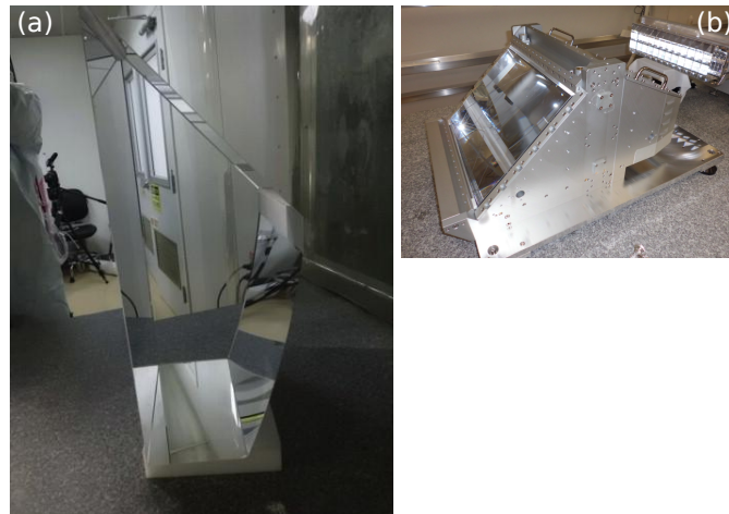
Fig. 5.8: (a) The FBLOCK made of radiation hard fused silica (Corning 7980). (b) The FBLOCK enclosed in its aluminium box. (c) Coupling of the new wedge to the FBLOCK.
