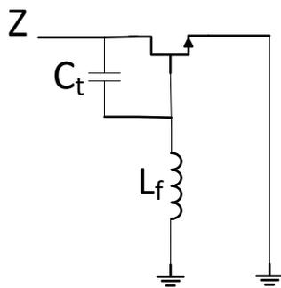
$$Z = \frac{1 - \omega^2 L_f (C_t + C_{gs})}{g_m + j\omega(C_t + C_{gs})}$$
