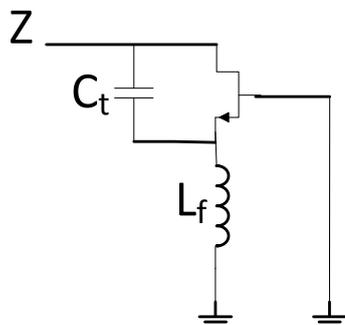
$$Z = \frac{1 - \omega^2 L_f C_t}{g_m + j\omega(C_t + C_{gs} - \omega^2 L_f C_{gs} C_t)}$$
