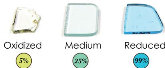
Figure 3 – Soda-lime silicate glasses (NCS) at three different redox states (oxidized, air synthesized, reduced), sample thickness: 2.5 mm.
