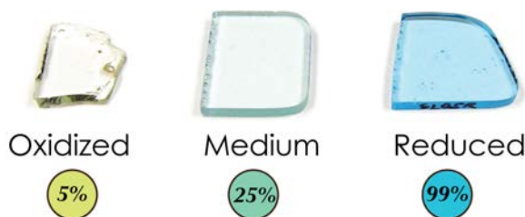
Figure 2.2 – Soda-lime silicate glasses (NCS) at three different redox states (oxidized, air synthesized, reduced), sample thickness: 2.5 mm.
