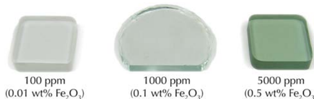
Figure 2.1 – Effect of iron content on diopside glass at 0.01, 0.1 and 0.5 wt% Fe 2 O 3 (size: ~2 cm, thickness: 5.5 mm).
