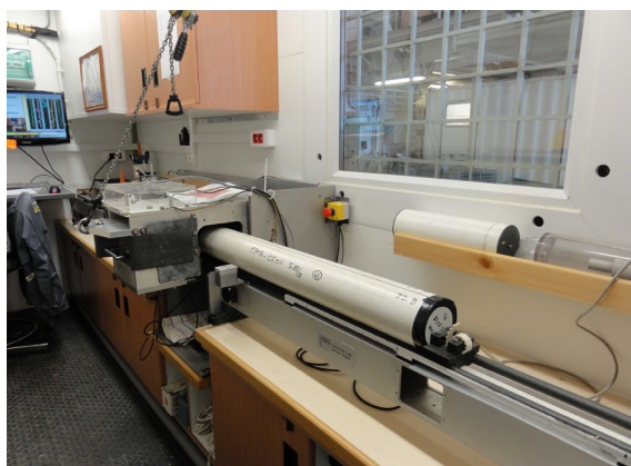
Fig. 2.5. GEOTEK Multi-sensor Core Logger (MSCL) in IFREMER container portable laboratory.
