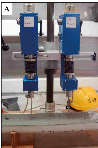
Fig. 2.9. (A) Photo of the IFREMER laboratory vane shear test with the vanes inserted in the sediment. (B) Example of an undrained shear strength ( Su ) curve obtained after a vane shear test. The maximum Su value corresponds to the peak shear strength and the value at 180^\circ of rotation after the peak corresponds to the residual shear strength.
