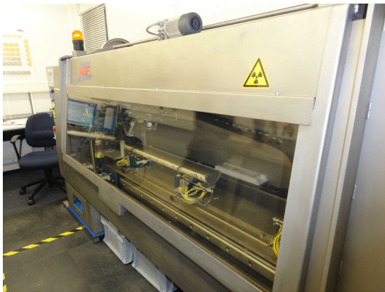
Fig. 2.7. Avaatech X-ray fluorescence (XRF) core scanner in IFREMER container portable laboratory.
