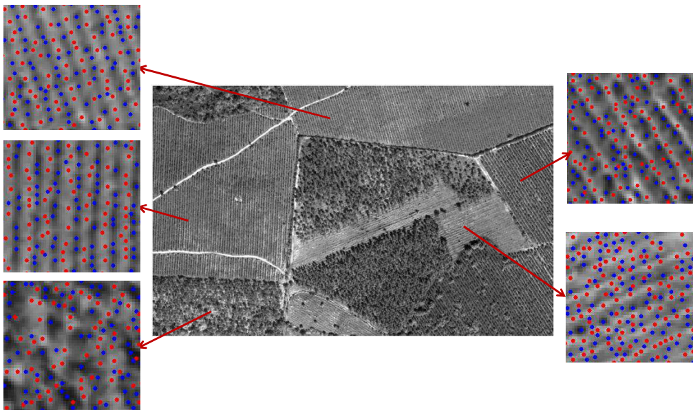
Figure 2.4 – Spatial distribution and arrangement of local maximum pixels (in red) and local minimum pixels (in blue) within different texture zones from a studied region of interest (ROI) of VHR panchromatic Pléiades image at 50cm resolution, ©CNES 2012, distribution Airbus DS/Spot Image.
