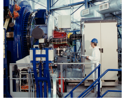
Figure 1.13 – NaCo instrument at the Nasmyth focus of the VLT-UT4 (before 2014). The NAOS system is within the light blue box and the Conica camera within the red box. Credit: ESO.
