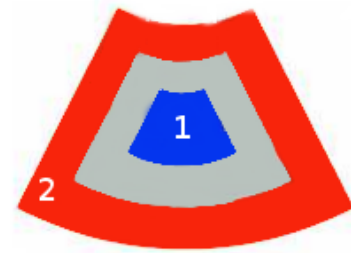
Figure 5.3 – Zone used to obtain the final image for TLOCI: The TLOCI coefficients are calculated for the zone in red (zone 2), whereas the subtraction is made in the blue zone (zone 1).
