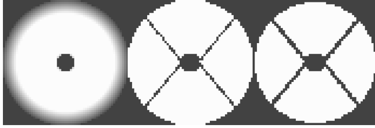
Figure 9.3 – Pupils used to produce the realistic simulated data. From left to right: Pupil apodizer (linear scale), upstream pupil and downstream pupil. The upstream and downstream pupils are binary masks generated from images of the pupils seen by the SPHERE-IRDIS detector.
