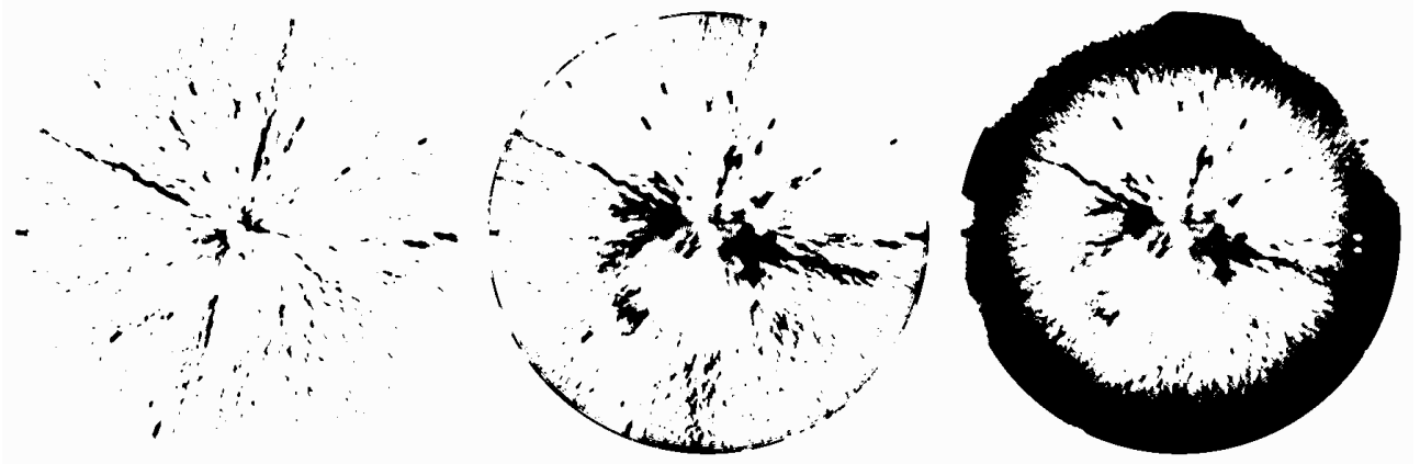
Figure 2.12 – SNR maps thresholded at 5\sigma , provided by ANDROMEDA using the parameters gathered in Tab. 2.4, using an empirical 2D-variance map. From left to right: without ADI optimization, with a total ratio optimization of the ADI and with a least-square optimization. Colors are inverted: white corresponds to zero and black to one.
