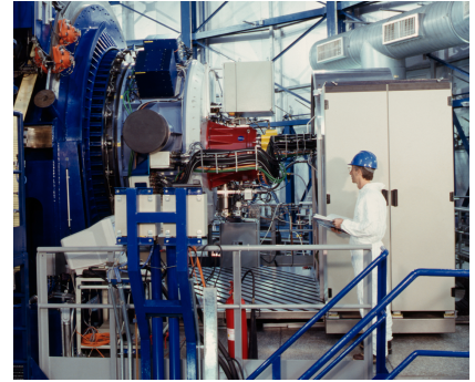
Figure 1.13 – NaCo instrument at the Nasmyth focus of the VLT-UT4 (before 2014). The NAOS system is within the light blue box and the Conica camera within the red box. Credit: ESO.
