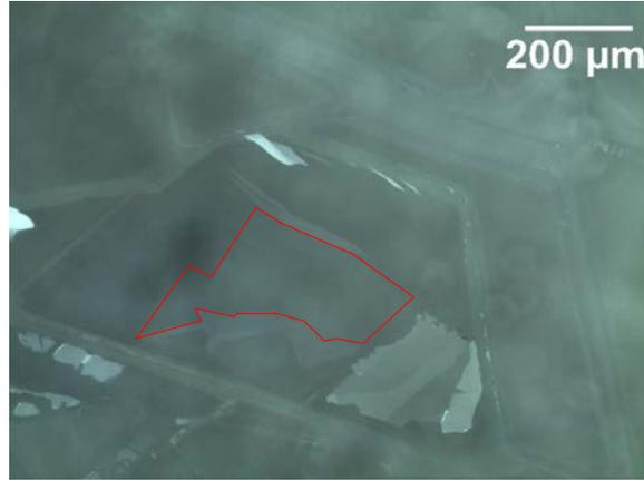
Figure 3.6: Optical image of a monolayer graphene sample on soda-lime glass (highlighted with the red line). The lateral size in one direction exceeds  $200\ \mu\text{m}$ .
