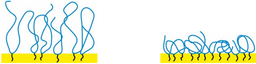
(a) Poorly grafted chains result in thick polymer layer.
