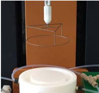
(a) Interfacial rheometer with "Double-wall ring" geometry. Ring and rheometer are provided by TA Instruments.
