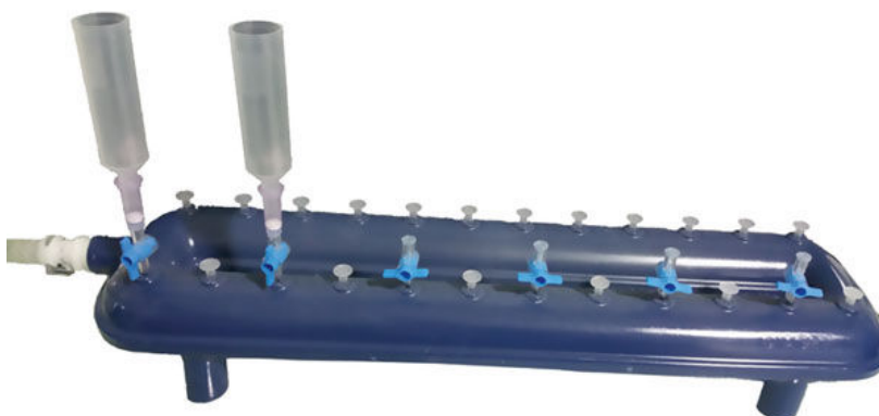
Fig. 2 Qiavac Manifold equipped with Qiaquick Spin columns and extenders to purify DNA from large-volume extracts
