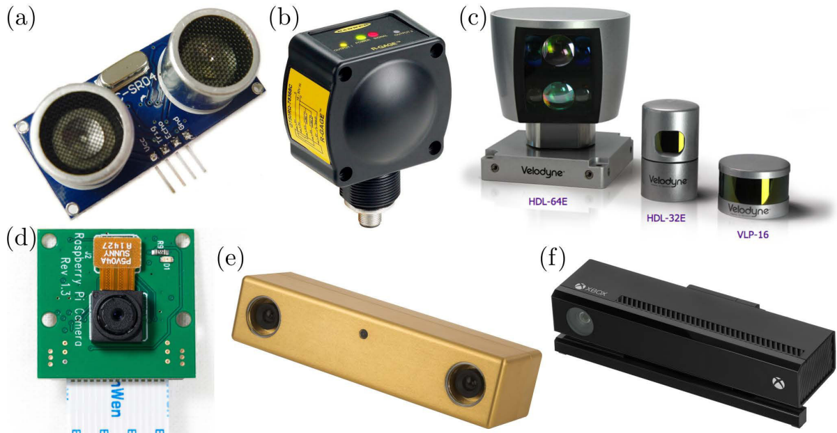
Figure 1.2: Example of sensors used in robotics and automobiles. (a) Ultrasonic sensor provided by Arduino. (b) Radar sensor provided by Banner Engineering. (c) Three types of lidars provided by Velodyne. (d) Camera provided by Raspberry Pi. (e) Stereo-vision sensor provided by Voltrium Systems. (f) Kinect camera (infrared depth camera) provided by Microsoft.
