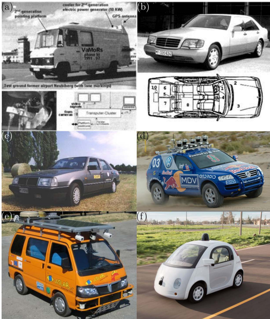
Figure 1.5: (a) The VaMoRs vehicle based on a Mercedes-Benz van, developed by Dickmanns’s research team at Bundeswehr University of Munich in 1986. (b) The VaMP vehicle based on a Mercedes 500 SEL, developed by Dickmanns’s research team at Bundeswehr University of Munich in 1994. (c) The ARGO vehicle based on a Lancia Thema, developed by the research groups of A. Broggi (University of Pavia, Italy) and C. G. Lo Bianco (University of Parma, Italy) in 1998. (d) The Stanley vehicle based on a Volkswagen Touareg, developed by the Stanford’s Racing Team, the winner of the DARPA Grand Challenge in 2005. (e) The driverless vehicle based on a Piaggio Porter, developed by the Artificial Vision and Intelligent Systems Laboratory (VisLab) at University of Parma, Italy for the Intercontinental Autonomous Challenge (VIAC) in 2010. (f) The Google Car, the first real-build driverless prototype vehicle delivered by Google in 2014.
