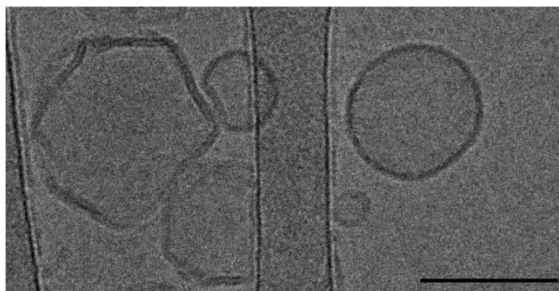
Figure 4.11. Cryo-TEM image of vesicles prepared from the 79/21 w/w % \text{PEO}_8 - b - \text{PDMS}_{22} - b - \text{PEO}_8 /DPPC mixture quenched from room temperature. Scale bar length is 100 nm.
