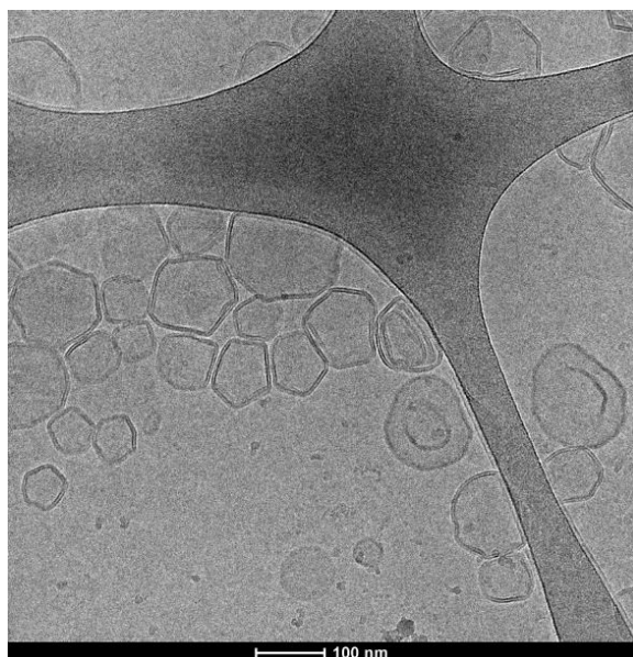
Figure 4.32. Cryo-TEM image of vesicles prepared from the 85/15 w/w ratio \text{PDMS}_{26}\text{-g-(PEO}_{12})_2/\text{DPPC} mixture quenched from room temperature.
