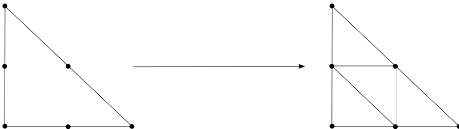
Figure 1.6: Action of OPERATOR LAGRANGE \mathbb{P}^1 on a \mathbb{P}^2 element in 2D. It transforms a \mathbb{P}^2 element into 4 \mathbb{P}^1 elements. The degrees of freedom are represented as black dots and the nodes of the elements are linked by black lines. The total number and the geometrical position of the degrees of freedom are not changed by this transformation.
