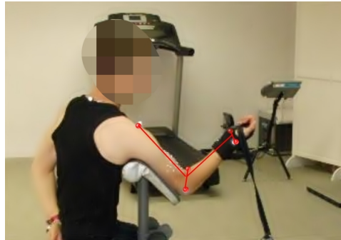
Figure 3.29: Elbow angle computing from the positions of the 5 markers placed on the acromion, the medial and lateral epicondyle, the radius and the ulna.
