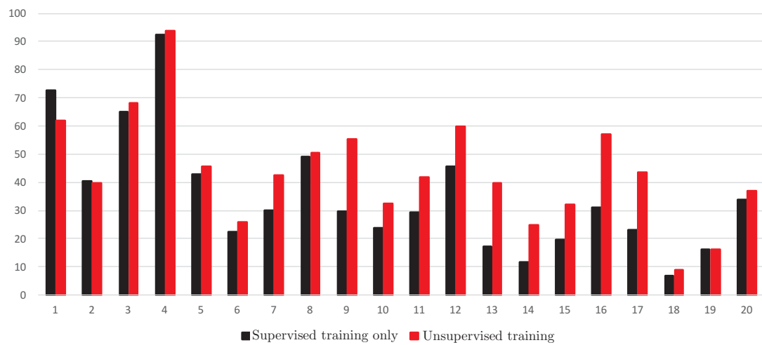
Figure 68 – Average segmentation accuracy per class obtained with the supervised method (in black) and after the unsupervised adaptation of the segmentation learner f_s(\theta_s) to the real data (in red). These results were obtained using our own dataset of real images. The horizontal axis shows numbers of hand segments (see Figure 63).
