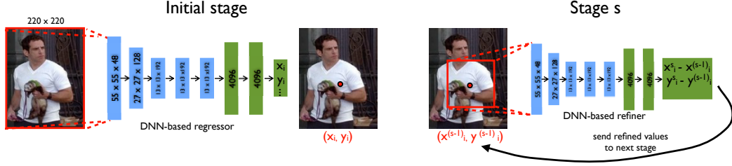
Figure 32 – Multi stage refinement of body pose estimation in DeepPose framework [297]. Convolutional layers are shown in blue and the fully connected layers are shown in green. The total number of stages in this implementation s \leq 3 .
