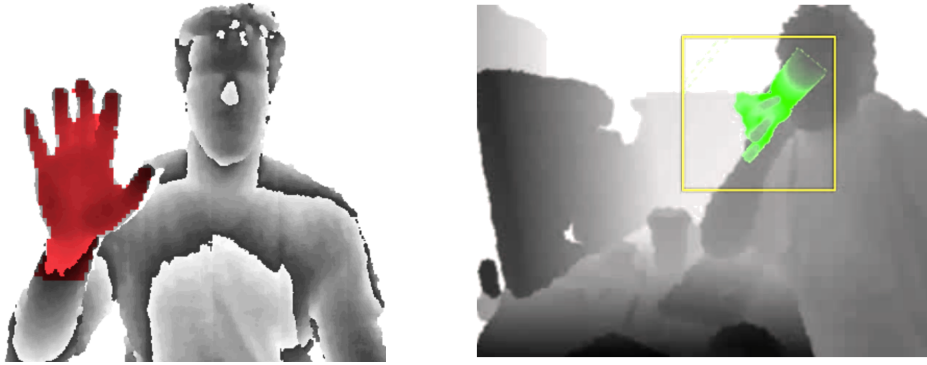
Figure 5 – An example of pixel-wise hand detection [296] (on the left) and of a failure case of hand pose estimation in a case of poorly segmented hand [134] (on the right). Figures are reproduced from the corresponding papers.
