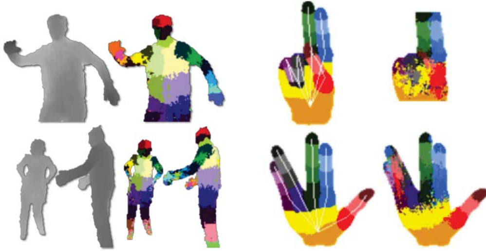
Figure 14 – Illustrations of depth-based body and hand segmentation methods, proposed in [266, 151] and based on classification random forests (RDF) (figures reproduced from the original papers). This segmentation step is typically followed by calculating pixel-wise votes for joint positions with a following aggregation stage.
