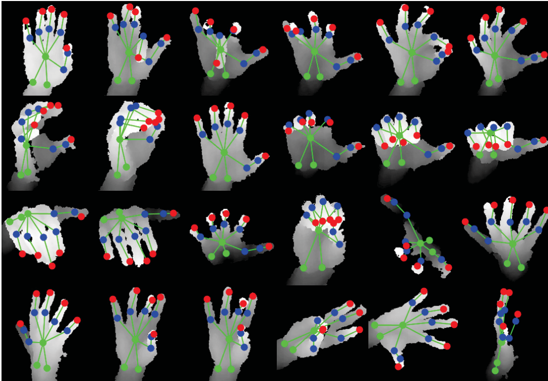
Figure 67 – Visualization of estimated hand skeletons produced by the regression learner f_r(\theta_r) . The regressor takes into account the intermediate representation produced by the segmentation network, which was tuned in a weakly supervised fashion.
