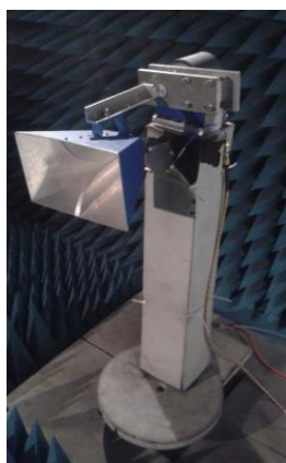
Figure 5.8 : Antenne de calibration.
