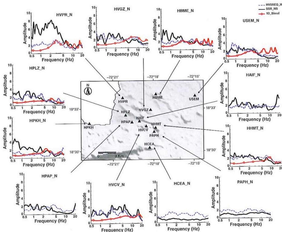
**Figure 9.** Comparison between SSR, HVEQ, and 1D equivalent linear (EQL) simulations (CyberQuake, Modaressi *et al.*, 1997). The black solid line shows the average SSR spectral ratios for the north–south component. The 1D simulation of soil seismic response is drawn in line with the empty circle and the HVEQ in the dashed line. The black triangles show the location of the seismic stations. The color version of this figure is available only in the electronic edition.
