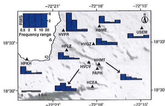
**Figure 11.** Root mean square (rms) diagram between the 1D numerical soil response and the computed SSR (north–south component) for different frequency bands ([0.5–2 Hz], [2–10 Hz], [10–20 Hz]). The black triangles show the location of the seismic stations. The color version of this figure is available only in the electronic edition.
