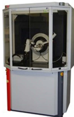
Figura II. 11. Difractómetro Bruker AXS Advanced X-Ray.
