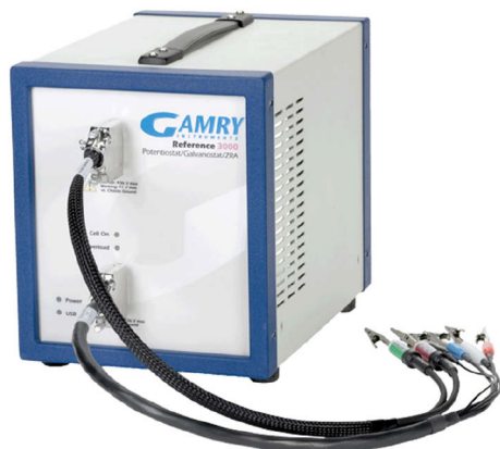
Figura II. 14. Potenciostato Gamry Reference 3000.
