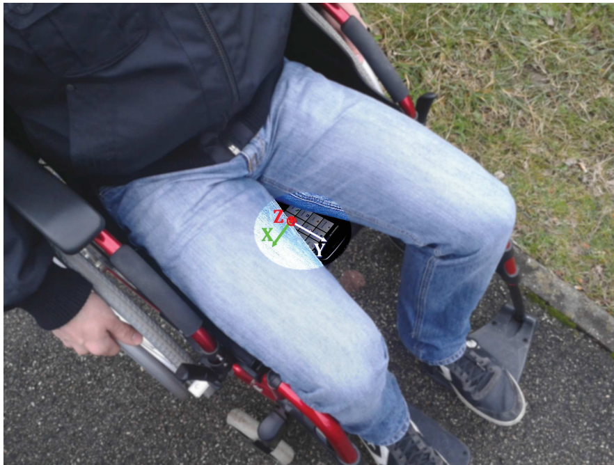
FIGURE 8.3 – Smartphone location and acceleration axes.
