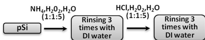
Scheme 1: Diagram illustrates the RCA1 and RCA2 protocols for porous silicon oxidation.
