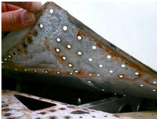
**Figure 1:** Degraded airplane piece demonstrating corrosion
