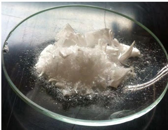
**Figure 2.4:** Very fine powder of boehmite nano-particles after freeze-drying
