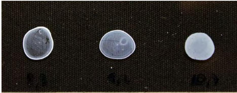
**Figure 4:** Dried droplets of an aqueous  $\gamma$ -alumina suspension for different  $pH$  values. The left deposit is an example of coffee ring formation, while the right one is a homogeneous deposit.
