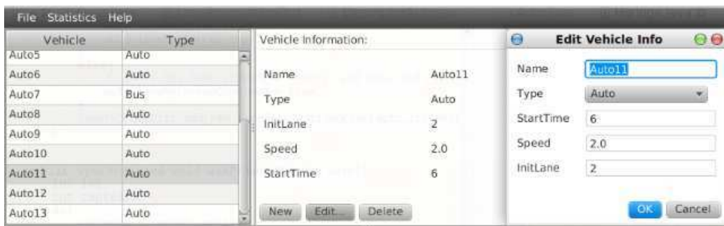
Figure 3.10: Traffic generator tool of the simulation environment
