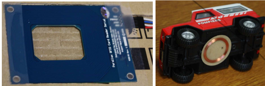
Figure 4.13: RFID reader and vehicle with RFID tag
