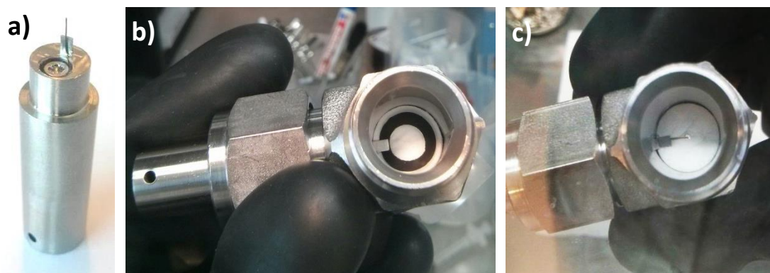
Figure 37: Photographs of the side current collector of a 3-electrode cell (a) and its utilization using a ring of self-standing LiFePO 4 (b) or a micro-electrode of Li touching a Cu wire (c) as reference electrode.
