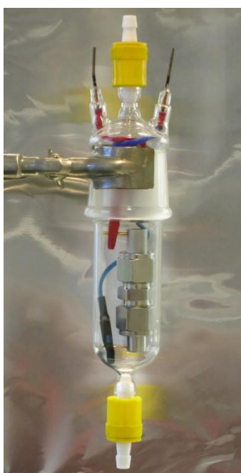
Figure 41: Photograph of a typical Li-O 2 cell used in the lab (handmade glass container ≈ 1200 €).
