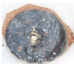
Figure 18. (Color online) Photograph of the Li anode surface after cycling.
