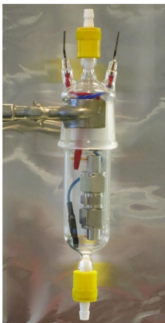
Figure 41: Photograph of a typical Li-O 2 cell used in the lab (handmade glass container ≈ 1200 €).
