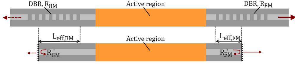
Figure 3-4: Schematic representation of the effective length of a DBR mirror (Top views of a laser).
