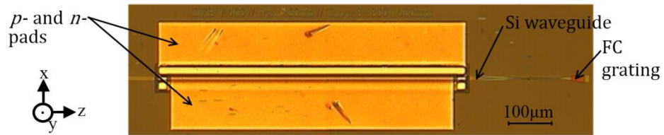
Figure 2-26: Optical microscope view of a DFB laser at the very end of the process.
