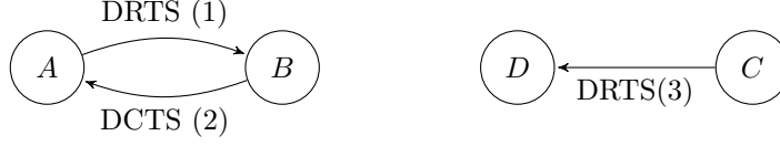
Figure 8.3: Hidden terminal (Case I).
