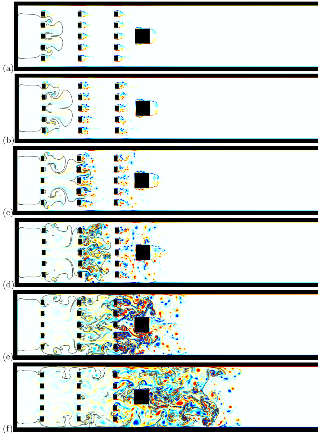
Figure 7.4: Snapshots of the vorticity field with iso-contours of the progress variable ( c = 0.2 and c = 0.8 ) that indicates the flame front for: (a) t = 4 ms, (b) t = 4.5 ms, (c) t = 5 ms, (d) t = 5.5 ms, (e) t = 6 ms and , (f) t = 6.5 ms. The red color corresponds to \Omega_z = 5 \times 10^4 \text{ s}^{-1} , while blue corresponds to \Omega_z = -5 \times 10^4 \text{ s}^{-1} . Simulation 2D-DNS1.
