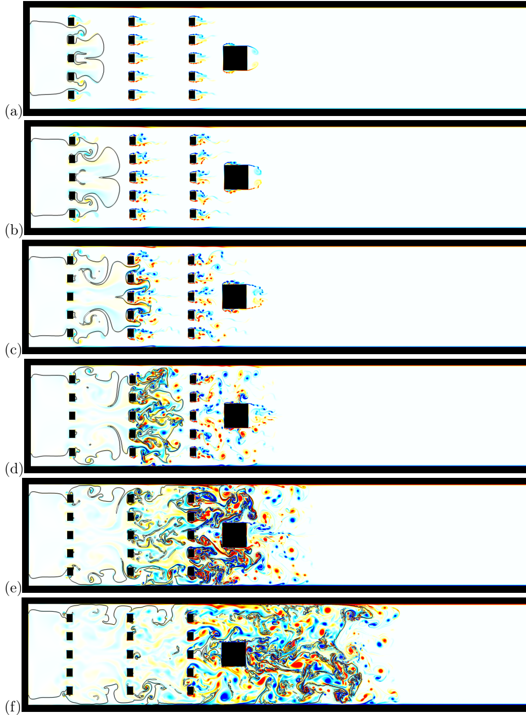
Figure 7.4: Snapshots of the vorticity field with iso-contours of the progress variable ( c = 0.2 and c = 0.8 ) that indicates the flame front for: (a) t = 4 \text{ ms} , (b) t = 4.5 \text{ ms} , (c) t = 5 \text{ ms} , (d) t = 5.5 \text{ ms} , (e) t = 6 \text{ ms} and , (f) t = 6.5 \text{ ms} . The red color corresponds to \Omega_z = 5 \times 10^4 \text{ s}^{-1} , while blue corresponds to \Omega_z = -5 \times 10^4 \text{ s}^{-1} . Simulation 2D-DNS1.
